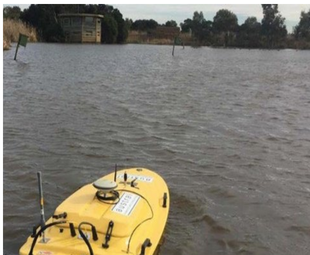
Figure MM10-4 Example of Benthic Monitoring using a Teledyne Oceanscience Z-Boat. (AECOM and GHD, 2018)
