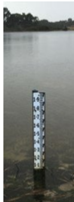
Figure MM10-5. Example surface water stage (level) monitoring. (AECOM and GHD, 2018)
