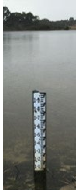
Figure MM07-2. Simple stilling well and Staff Gauge Setup (DRW, 2016).
