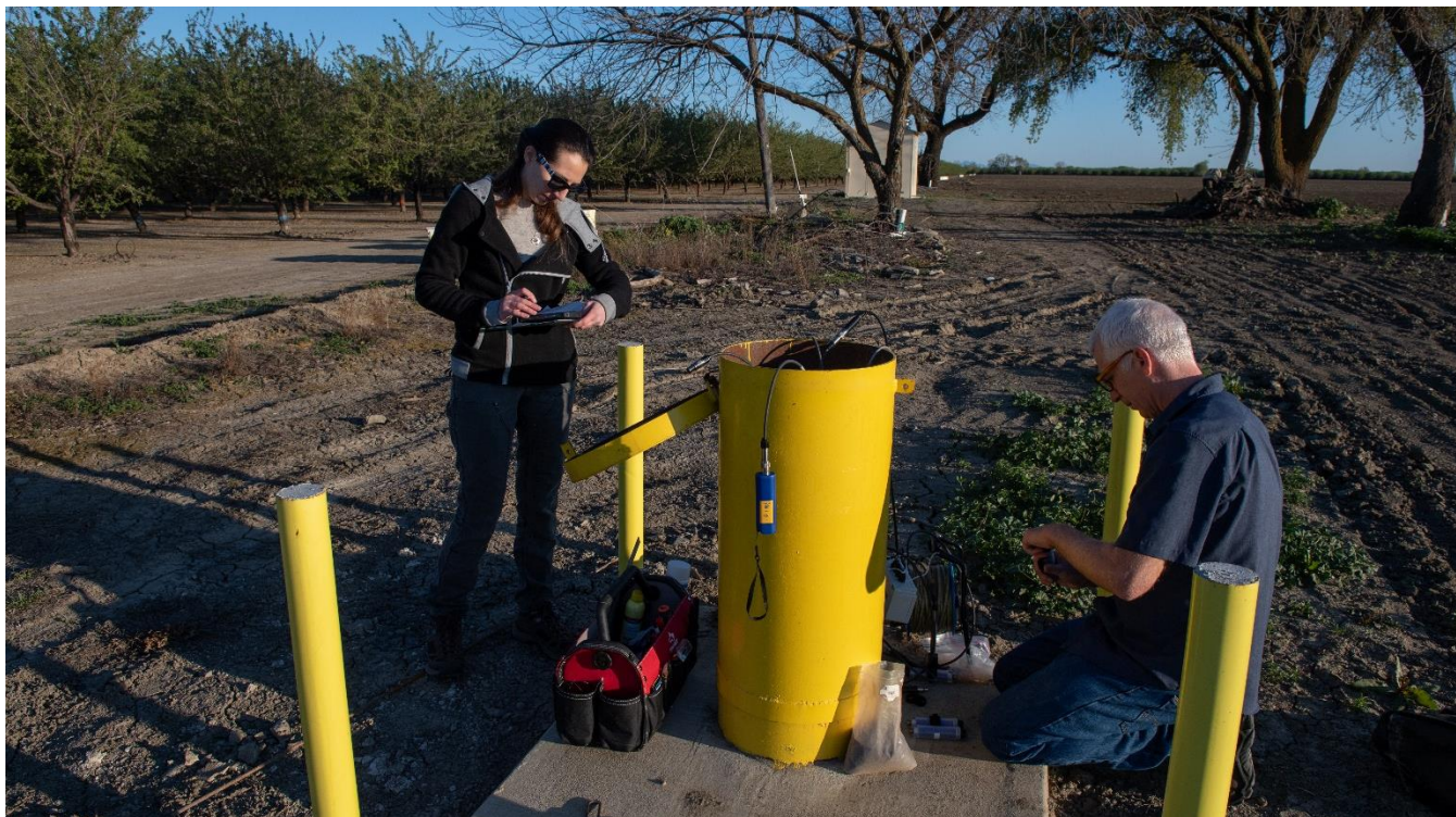
Photo 2: DWR Staff Measure the Groundwater Level in a Monitoring Well Located North of Sacramento, California.
