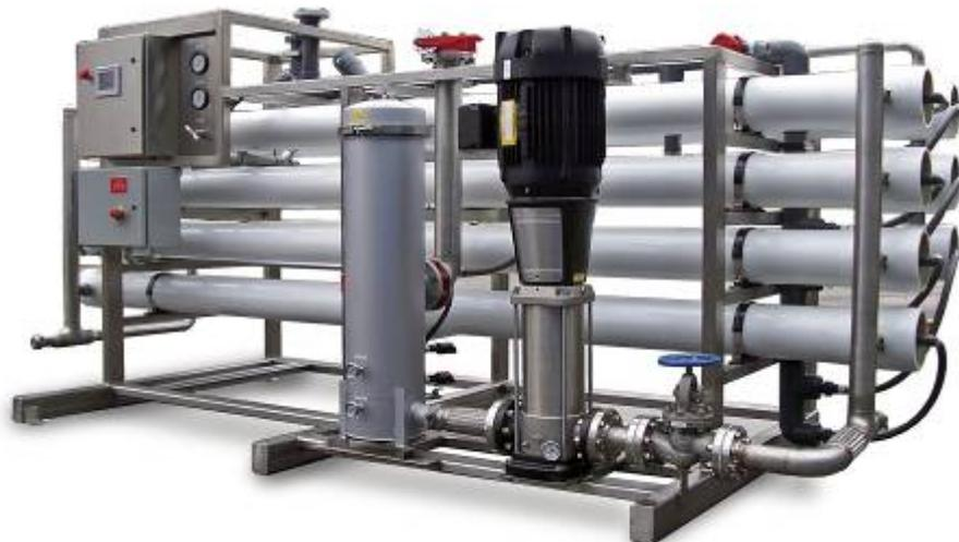
Skid-mounted Reverse Osmosis Mobile Water Desalination Unit
