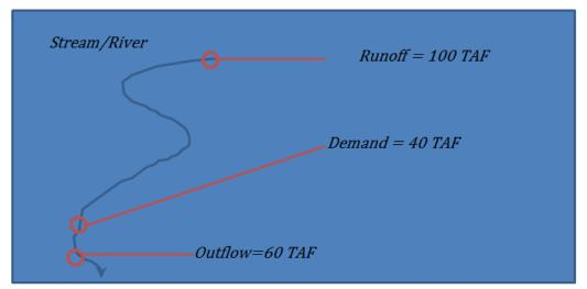
Figure A-SW9. WEAP Outflow Concept
