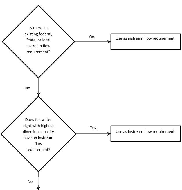
Figure A-SW1. Instream Flow Requirement Approach
